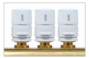
**Image 4:** Möhlenhoff's portfolio includes the Smart Valve Drive with a stroke of 3.5 millimeters and actuating force of 90 Newtons for installation in confined spaces.
