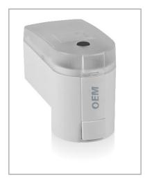
**Image 5:** The Motoric Valve Drive motoric actuator has a stroke of 8.5 millimeters and is available with actuating forces of 100, 125, 150 and 200 Newtons.
